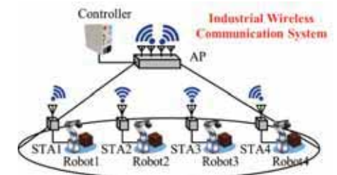
Industrial wireless LAN system (system configuration)
