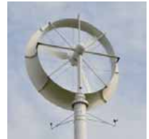
3 kW lens windmill (single machine), Kyushu University Ito Campus installed, and about 10 other turbines (independent system)
