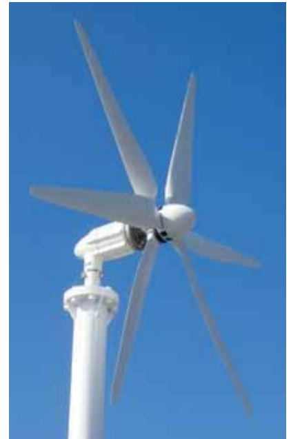
1 kW (2.2 m diameter) wind turbine currently in operation in Higashi-ku, Fukuoka-shi and Kurume-shi
